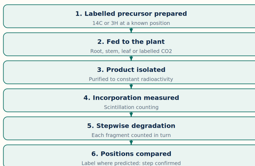
Figure: The radio tracing workflow. Purification to constant activity and the degradation step are what separate a proof from a suggestion.
