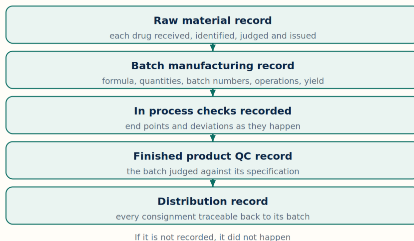
Figure: The documentation chain. Every batch carries its own paper life, from the raw material verdict to the consignment that can be traced back to it.
