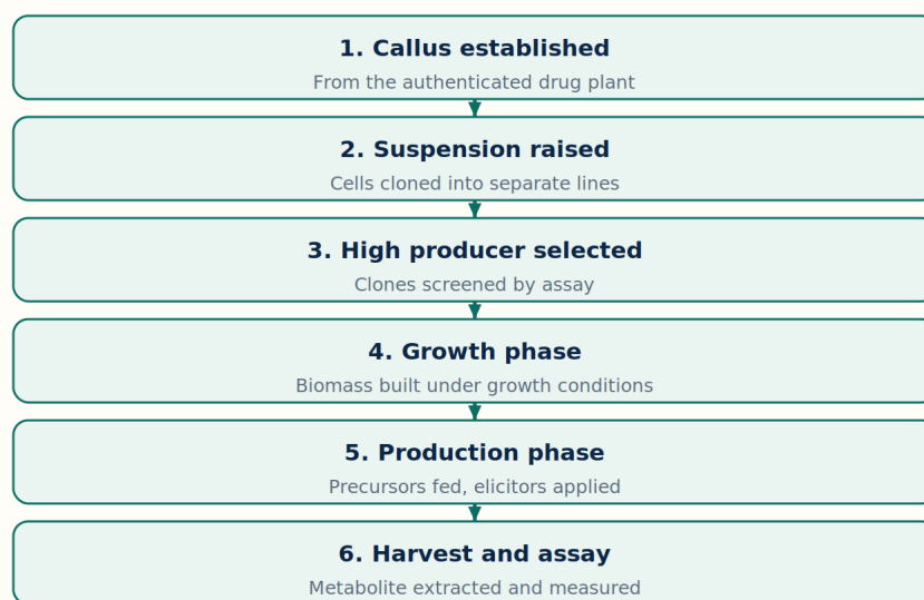
Figure: From callus to metabolite. Selection finds the producing line; the separate production phase, with precursors and elicitors, is where the yield is actually made.
